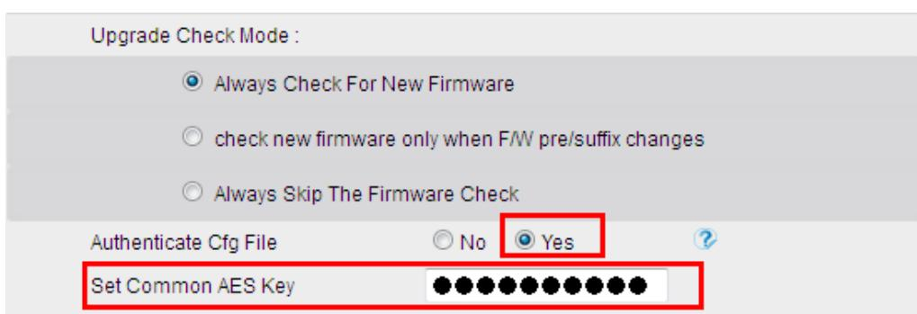
The common AES key can be configured using the configuration file and web interface.
