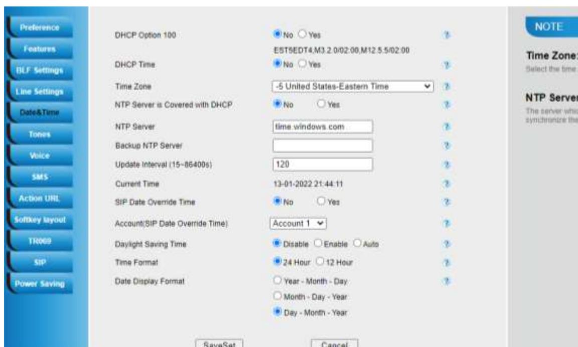
The screenshot shows the 'Date & Time' configuration page in a web interface. On the left is a navigation menu with options: Preference, Features, BLF Settings, Line Settings, Date & Time (selected), Tones, Voice, SMS, Action URL, Softkey layout, TROOP, SIP, and Power Saving. The main content area contains the following settings:
