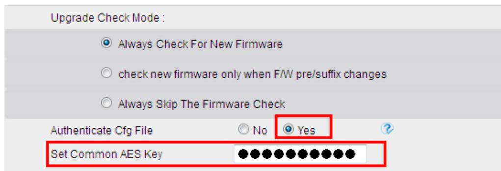
The common AES key can be configured using the configuration file and web interface.
