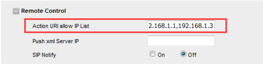
The screenshot shows the 'Remote Control' configuration section. The 'Action URI allow IP List' field is highlighted with a red box and contains the text '2.168.1.1,192.168.1.3'. Below it, the 'Push xml Server IP' field is empty. The 'SIP Notify' option is set to 'Off'.
